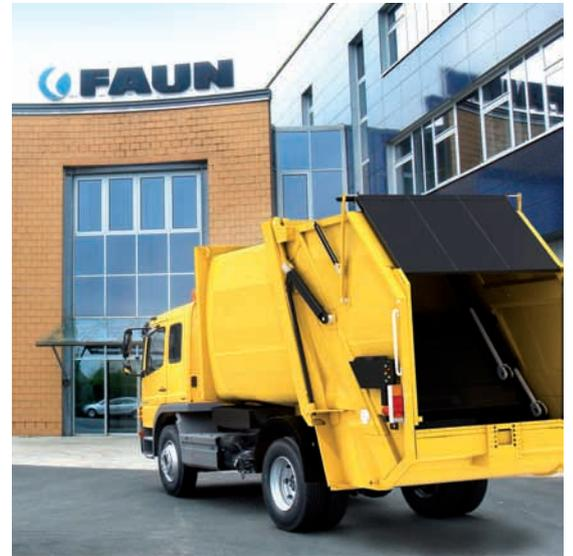
FAUN VARIOPRESS 2.30 m wide on twin-axle chassis
