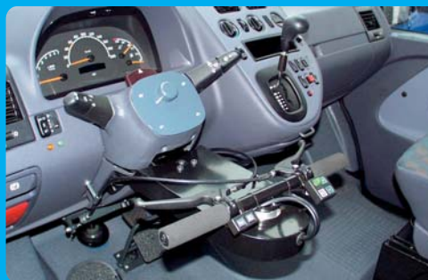
Steering aid, here using motorcycle handlebars
