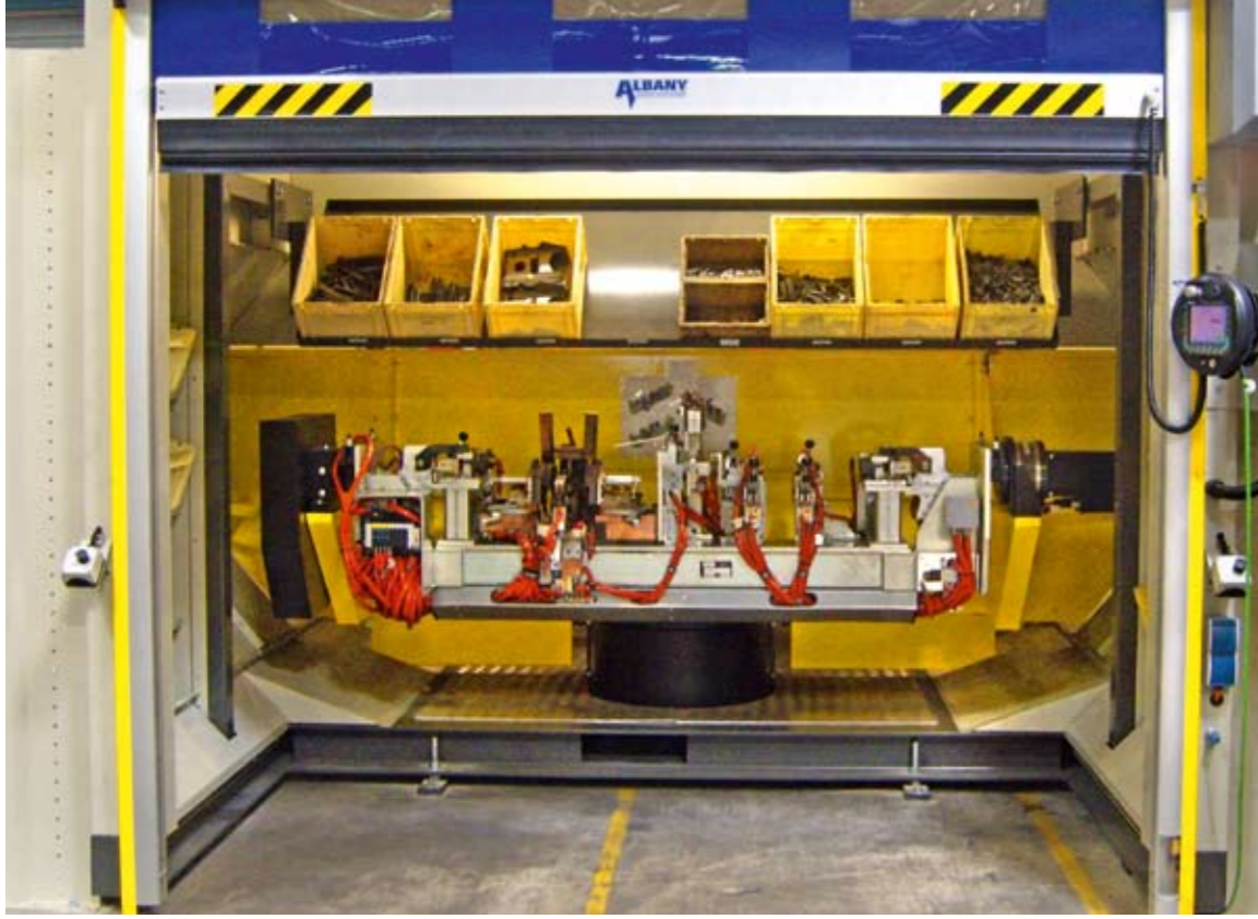
Welding cell for the new Peugeot cross car beam
