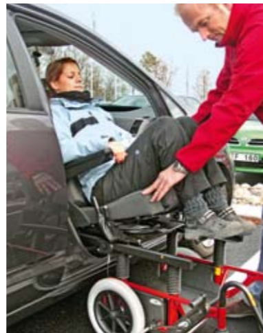
The swiveling car seat „Tilda“ can be tilted back up to 15 degrees
