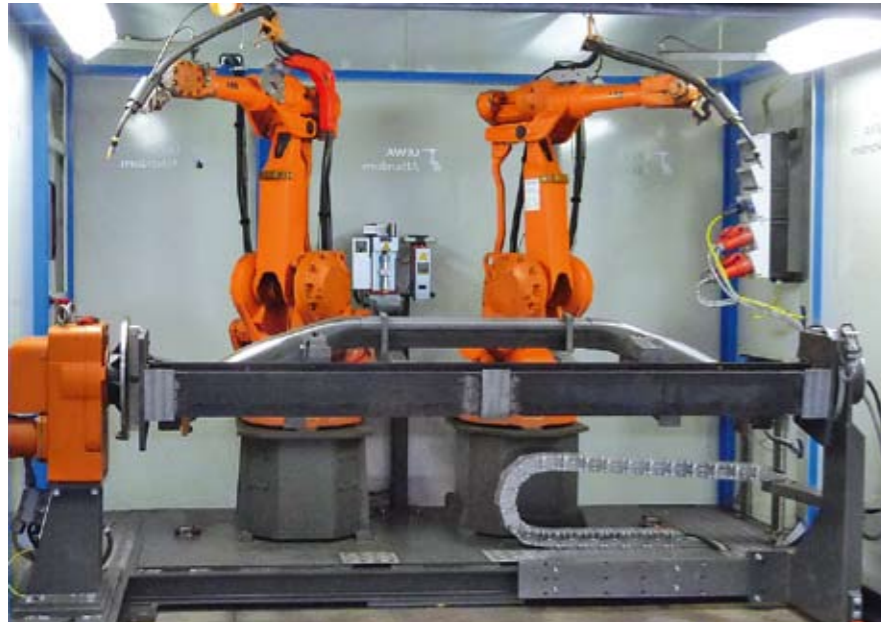
Robot cells equipped with the most modern equipment for MAG welding processes work on prototypes and pre-series parts using the arc-welding process
