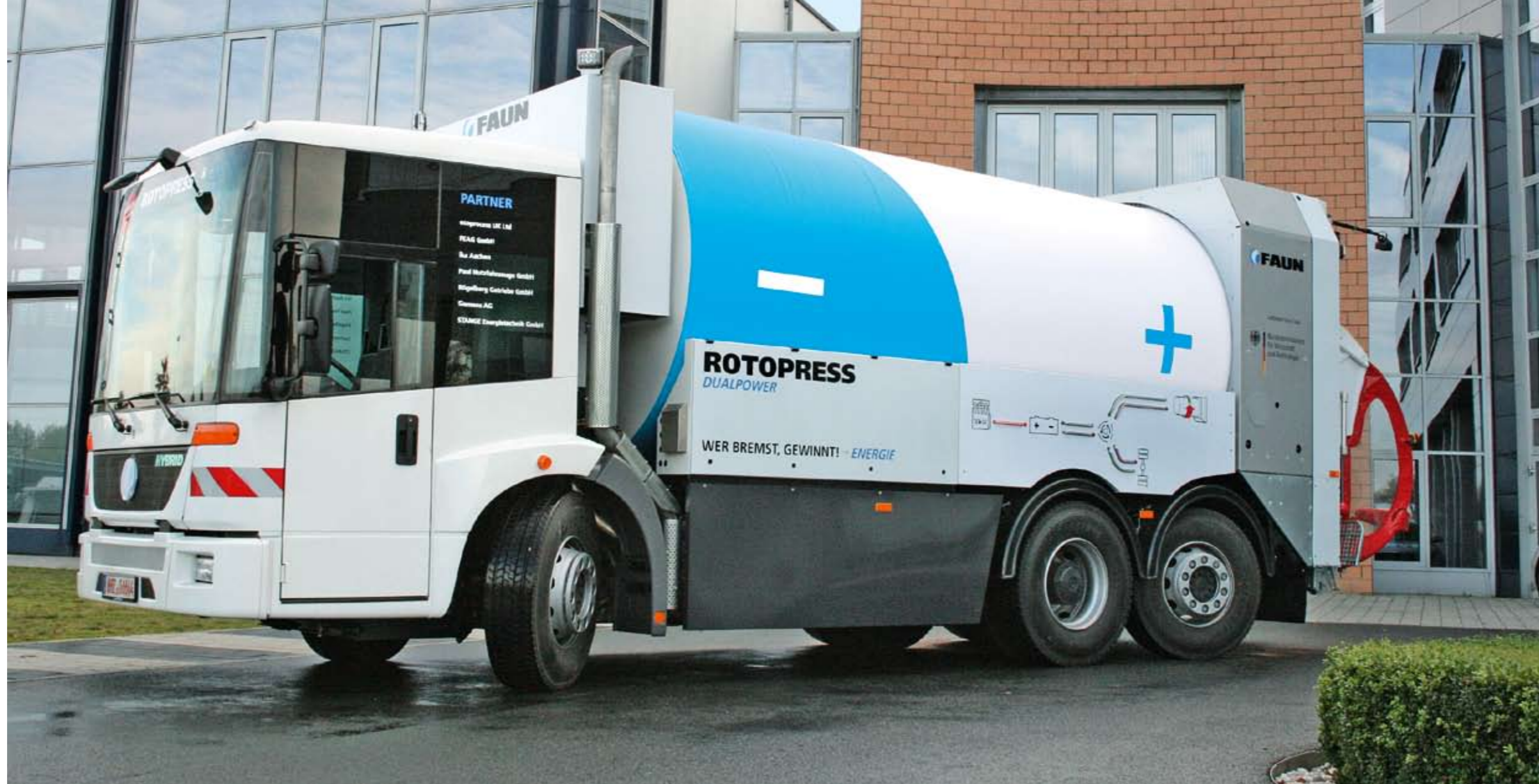
FAUN ROTOPRESS DUALPOWER with diesel-electric hybrid drive
