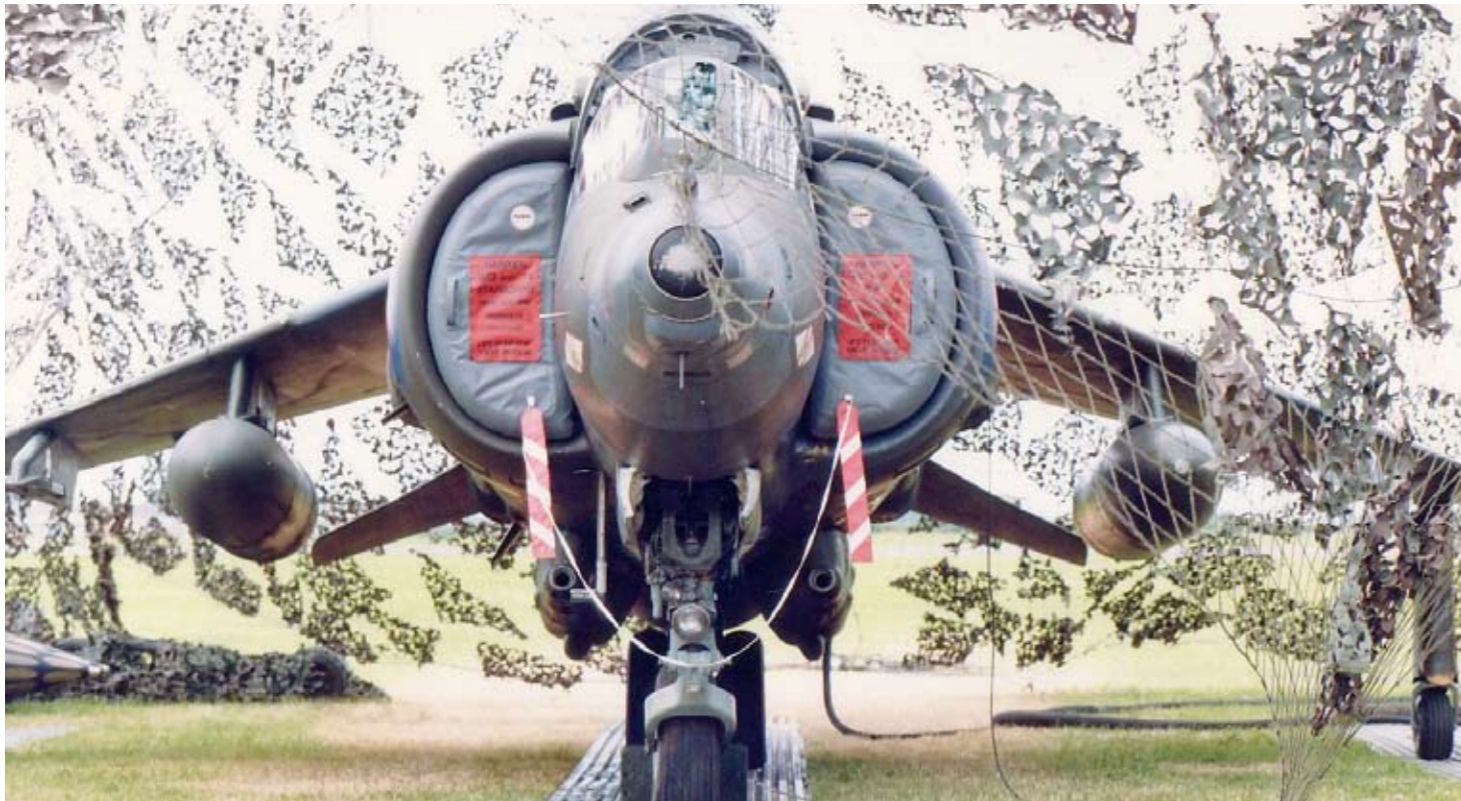
Harrier utilising the old style PSA panels as a temporary hard standing
