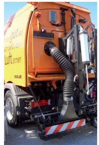
The detachable rear suction unit creates a sweeping width of 2.30 m.
