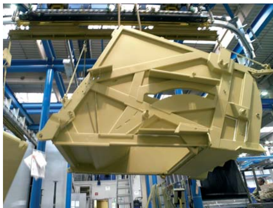
The body parts are painted in one of the cabins immediately after the grinding.
