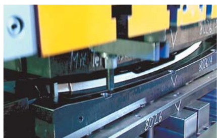
4. Prototyping: initial product manufacture – here pressing
