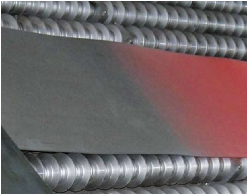
Partially tempered blank
